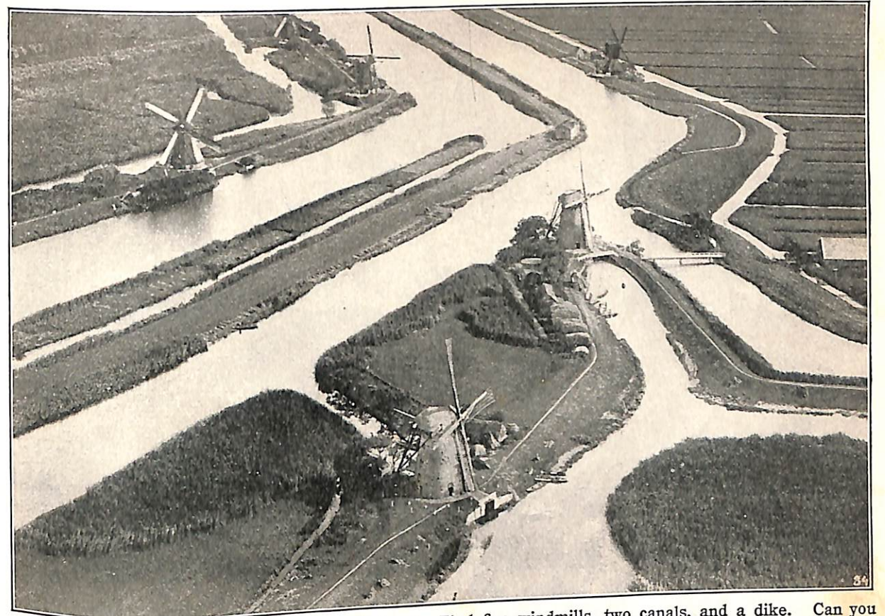
Fig. A. An air view of the polder lands in Holland. Find five windmills, two canals, and a dike. Can you see where water is lifted from one canal into another?
