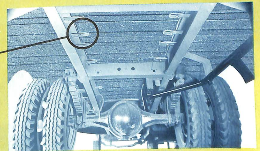
A thorough rubberized coating is sprayed on the underfloor for insulation and additional rust prevention
