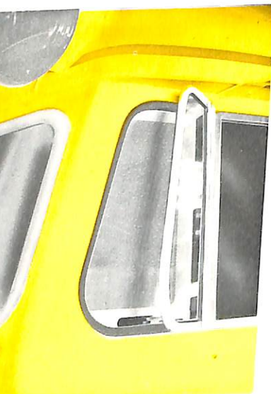
BLUE BIRD'S EXCLUSIVE screened driver's vent. Easy to operate from inside.
