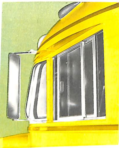
Outside full-length rear view mirror on adjustable brackets is easy to reach through sliding window.
