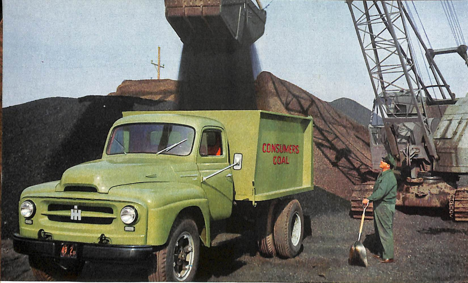
Above: Model R-184 LOADSTAR, 142-inch wheelbase, with 8-yard coal body. Steel-flex frames proved best in the field. Cushioned disc clutch. Gross vehicle weight rating 21,500 pounds. Color: Door County Green.
