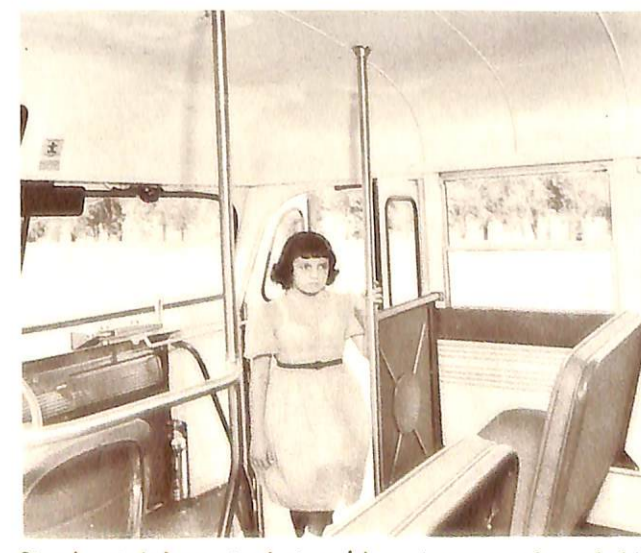
Sturdy stainless steel stanchions increase safety of children entering or leaving bus. Tubular rail behind driver's seat
