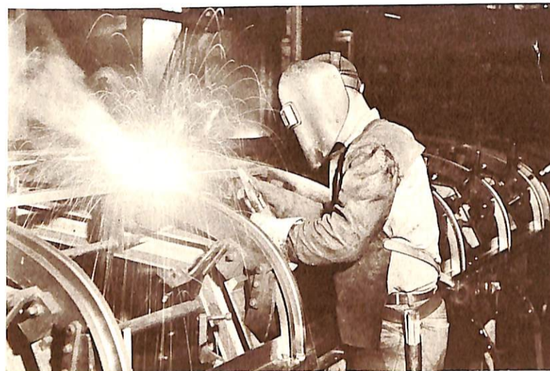
Steel welds steel for utmost strength as the roof frame members locked in this precision jig are all welded into one complete unit. Sturdy, one-piece roof bows assure maximum strength in event of a roll-over.
