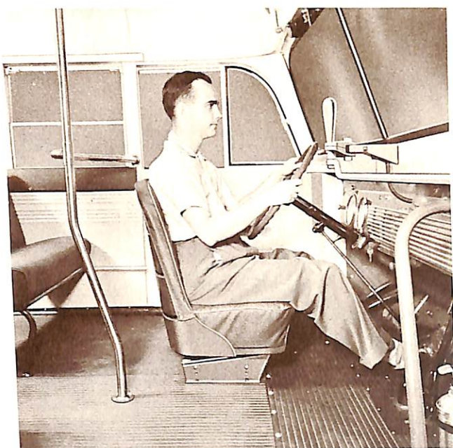
Instantly adjustable driver's seat gives best eye-level and driving position for each individual; moves on track—forward and up for shorter driver, backward and down for taller driver. Heavily padded, form-fitted back; resilient spring-type cushion; durable, plastic-coated trim.
