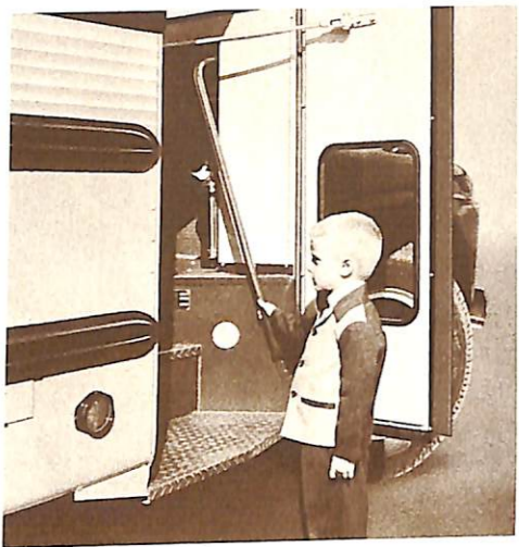
Easy-to-reach hand rail helps even the smaller children get on or off safely. Non-slip steps. Automatic step-well light.
