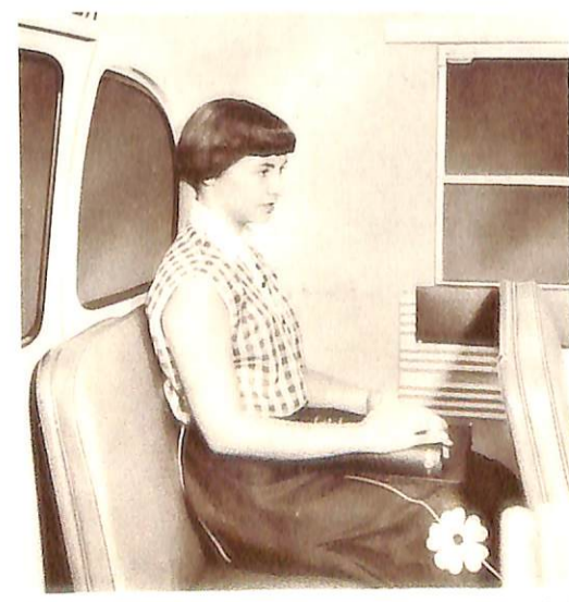
Extra headroom at rear eliminates "bent-neck" posture, cuts down possibility of head injury from
