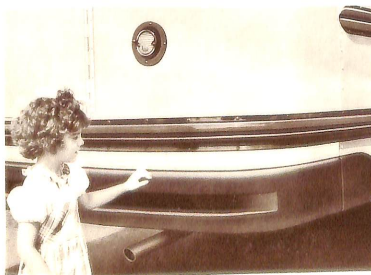
Super protection at rear where buses are most often hit: massive, box-section steel pillars, roof-mounted, optional
