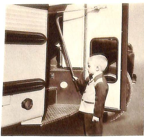
Easy-to-reach hand rail helps even the smaller children get on or off safely. Non-slip steps. Automatic step-well light.
