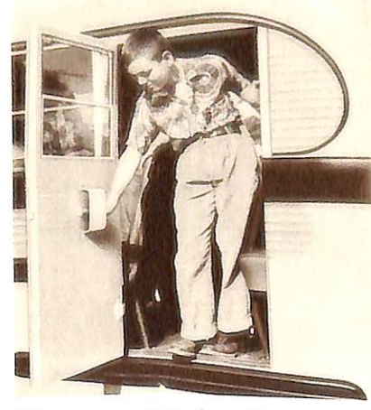
Side emergency door blends with exterior styling. Same type hinge, double catch, release guard, and rubber seal as rear door. Available when specified.
