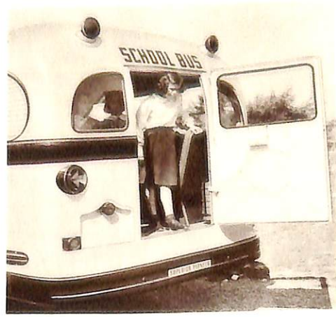
Rear emergency door swings on piano-type hinge; rust-proof pin. Double catch for extra safety. Guard over inside release. Rubber sealed.
