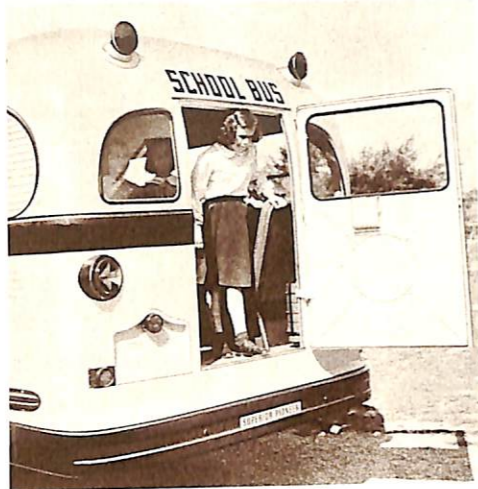
Rear emergency door swings on piano-type hinge; rust-proof pin. Double catch for extra safety. Guard over inside release. Rubber sealed.
