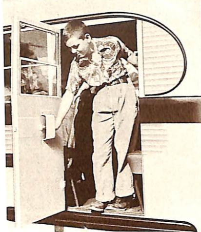
Side emergency door blends with exterior styling. Same type hinge, double catch, release guard, and rubber seal as rear door. Available when specified.
