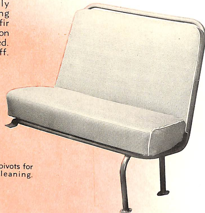
Seat backs are tapered for increased aisle clearance.
